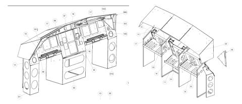
1.2 Arrange the four legs following the sample image and screw the rear trays and the central reinforcement bar.
